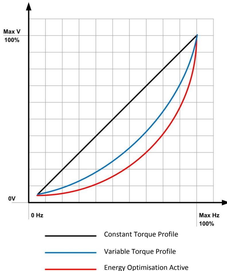
It can be seen that energy savings exist in the area between the different profiles. The Energy Optimisation function adjusts voltage to provide energy savings under all conditions. Even a constant torque drive with energy optimisation function can operate the motor more efficiently than a variable torque drive without energy optimisation.
