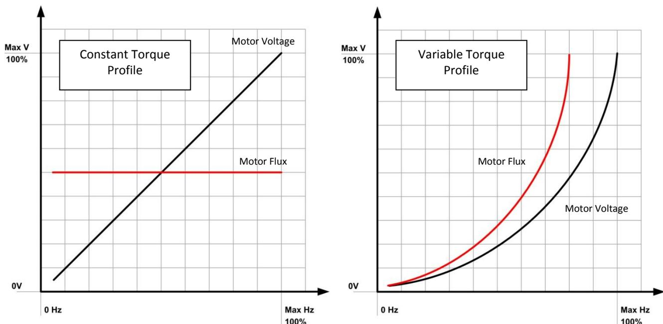
As its name implies, the constant torque voltage profile provides the best results in terms of energy saving when the load is constant and close to its nominal value. But under no load conditions the excess in magnetizing current would unnecessarily increase the losses in the stator making the motor less efficient.
