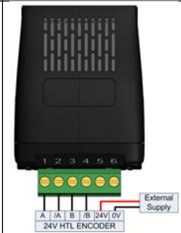
Connection Example – 24V HTL Encoder OPT-2-ENCHT-IN
