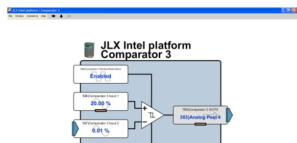
The threshold for DIO1 operation is set by 596)Comparator 3 Input 1, and hysteresis by 599)Comparator 3 Hysteresis.
