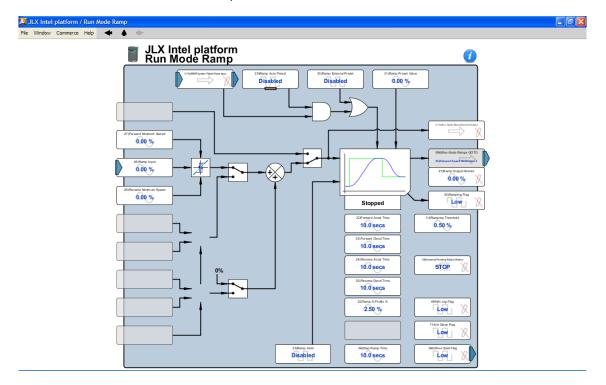
The settings required here are 22)Forward Accel Time, 23)Forward Decel Time, 24)Reverse Accel Time and 25)Reverse Decel Time. An S profile may be introduced if desired. These ramp times come into effect in response to a change of analogue speed demand on T4. Please note that the times entered will be those pertaining to a 100% change in demand. Use the back arrow to return to the block diagram page then left click on the Stop Mode Ramp block.
