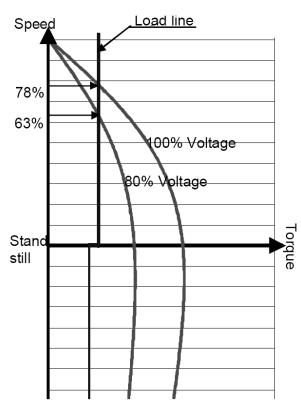
The curved lines represent the Speed / Torque relationship at 100% and 80% Stator voltage.
