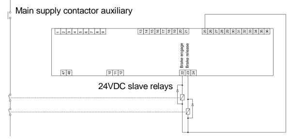
Brake supply outgoing Supply off = brake engaged
