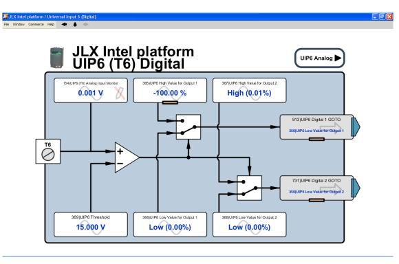
and set 365)UIP6 High Value for Output 1 accordingly (remembering this value has to be negative).
