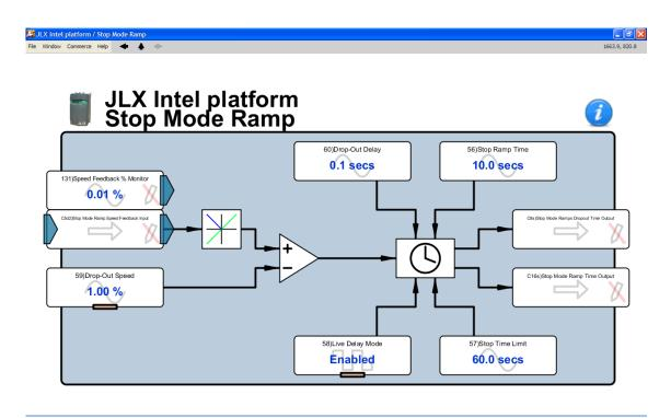
56)Stop Ramp Time is set here – usually to the same time as the previously set Run Mode Ramp times. This setting comes into effect when opening T33 (Start terminal) or (if used) the Start Positive or Start Negative terminals (T5 and T6).
