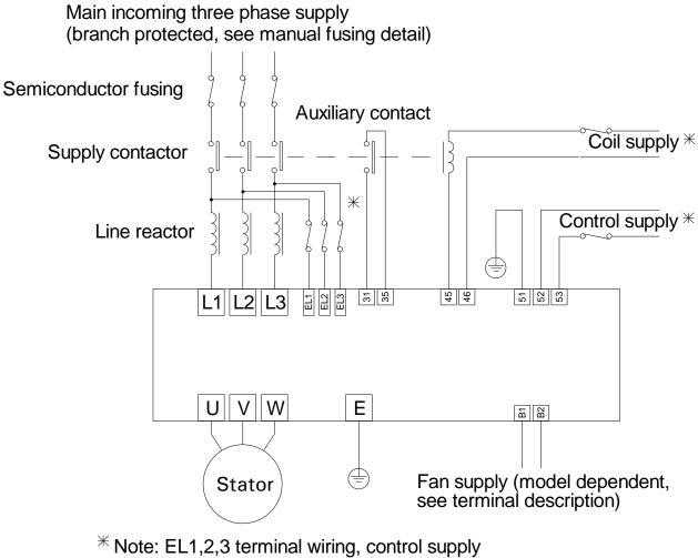
\* Note: EL1,2,3 terminal wiring, control supply and coil supply breaker or HRC fuse protected 5.2 Basic analogue bipolar input speed control (as shipped, default configuration)
