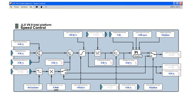
If necessary, reduce the value of 72)Speed Integral Time Constant so that the speed follows the step change in speed demand as closely as possible. Then return to the block diagram page containing the Speed Control block, left click on the Parameter Profiler block
