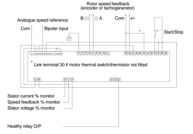
5.3 Basic analogue unipolar input speed control (as shipped, default configuration)
