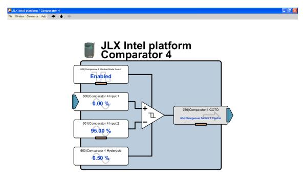
The threshold for sensing intentional hyper-synchronous operation is set by 601)Comparator 4 Input 2, with hysteresis set by 603)Comparator 4 Hysteresis. The setting is to be just less than the maximum demand available from UIP4, set previously.
