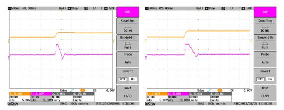
The picture on the left shows current demand peaking at about 150% which is acceptable. The picture on the right shows a larger speed demand step change forcing the current demand to saturate and clamp at 150%, which is not acceptable for speed loop tuning purposes.
