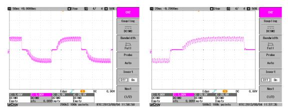
**Important note:** The maximum average level observed on the oscilloscope trace will be scaled according the ratio of your setting for 2)RATED STATOR AMPS against the maximum current capability of the JL/X model in use. The
