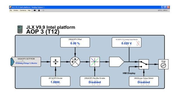
Delete the 929)AOP3 GETFROM connection and connect instead to 718)Unfiltered Current Demand Monitor. Also set parameter 257)AOP3 Divider to 2.0000.
