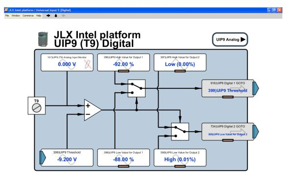
The negative hyper-synchronous detection level is set by 399)UIP9 Threshold. For example, a desired hypersynchronous detection level of -90% speed (i.e. -90% of the previously set value for 6)Desired Maximum RPM) requires 395)UIP9 High Value for Output 1 to be set to approximately -92.00% and 396)UIP9 Low Value for Output 1 to be set to approximately -88.00%.
