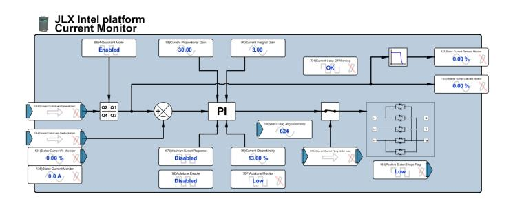
Right click on the 90)Current Proportional Gain parameter and select "Add to Parameter Dock". Repeat for the 94)Current Integral Gain and 95)Current Discontinuity parameters. Navigate to the dock page, which should now appear similar to this.
