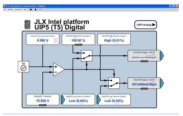
and set 355)UIP5 High Value for Output 1 to the previously calculated scaling factor.
