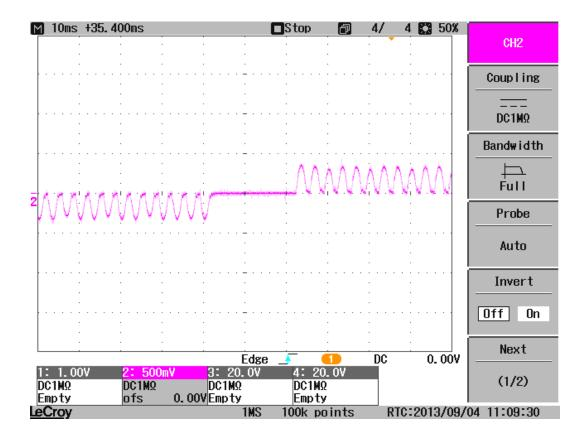
If a reasonable minimum "dead time" (say minimum of 6 to 8mS) is not observed because the stator is highly inductive please see later section 6.4.3 Special techniques for highly inductive stators.
