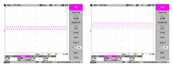
Discontinuous current is where the current pulses are discrete and have portions between them sitting on the 0V datum (left hand picture). Continuous current is where the current pulses join together and lift away from the 0V datum (right hand picture).
