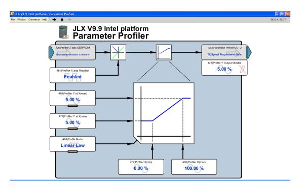
and increase both 477)Profiler Y at X(min) and 478)Profiler Y at X(max) values to damp out any overshoot observed. The following picture shows a correctly tuned speed loop.
