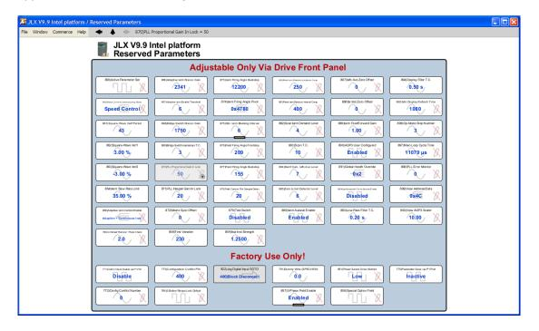
Setting this parameter to ENABLED has a \*10 scaling effect on 93)Current Proportional Gain – so that (for example) entering a value of 3 will result in an applied value of 30. It also disables INTERNAL ERROR CODE 0005 as this is inappropriate for very long time constant loads. It is also necessary with highly inductive stators to allow an extended "dead time" around zero current setting. To do this, navigate to the block diagram page containing the Current Monitor block
