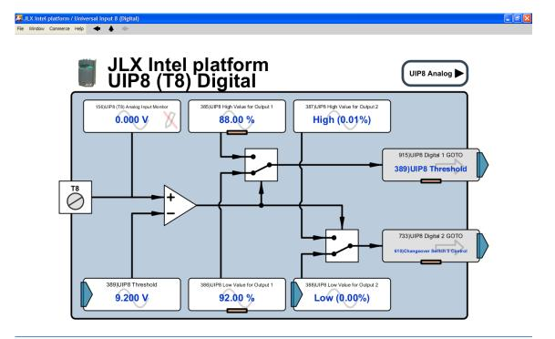
The positive hyper-synchronous detection level is set by 389)UIP8 Threshold. This in turn is set by 385)UIP8 High Value for Output 1 and 386)UIP8 Low Value for Output 1. The values for these parameters should be set symmetrically around the desired hyper-synchronous detection level in order to provide hysteresis. For example, a desired hyper-synchronous detection level of 90% speed (i.e. 90% of the previously set value for 6)Desired
