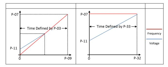
It is important to understand this alternative approach to motor starting in order to correctly commission the drive. Note that once the motor is started, a linear V/F characteristic is used during control, from 0 Volts, 0 Hz to Rated Volts, Rated Frequency.
