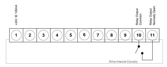
Note that when the drive is powered down, the contacts are always open.
