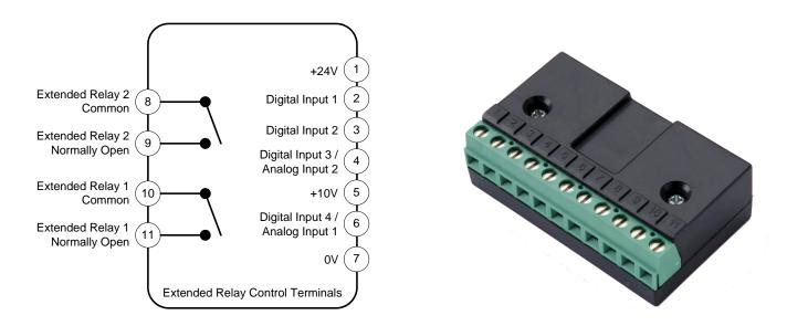
The Option module is fitted to pins 1 - 11 on the drive control terminal block of the Optidrive E2.
