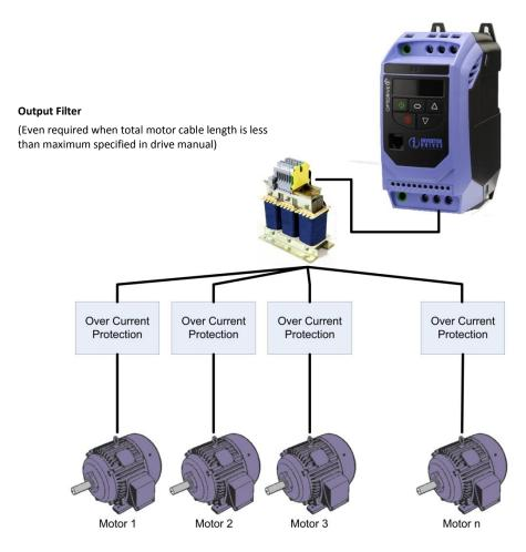
With this connection method individual motor cables are run between the drive and each of the motors with a common connection (star) point located close to the drive. Over-current protection for this configuration is typically located near to the drive so that each motor cable down-stream from the over current protection device is rated only for the motor it protects.
