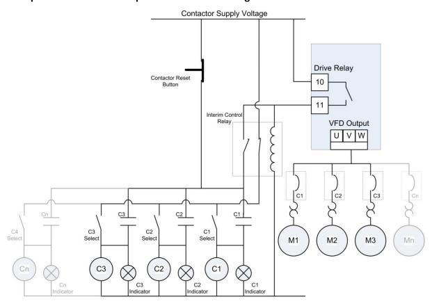
This circuit requires an additional interim relay in addition to the drive user relay in order to provide normally open and normally closed contacts for the successful operation of the circuit.
