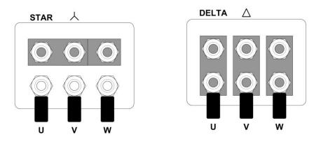
87Hz operation exploits the possibility that the motor could be configured for low voltage 230V (Delta) operation but actually be supplied from a 400V source / drive. In effect the maximum voltage applied to the motor terminals has been increased by a factor of root (3). To avoid over fluxing the motor and to provide a constant Volts/Hz ratio the nominal motor frequency should also be increased by root (3) resulting in the 87Hz operating point.
