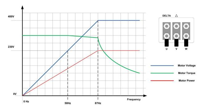
There is some Torque reduction above 50Hz caused by the increased iron losses that result from operation at a higher frequency but the net result is a significant increase in the power output from the motor.
