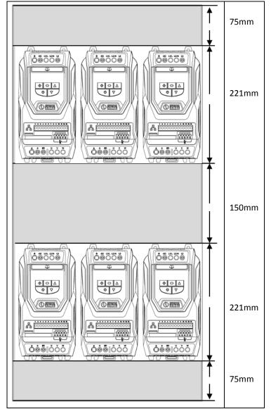
In both the above examples, the grey shaded areas above and below the drives are to be left free to allow air to easily enter and exit the drive cooling channel. No equipment may be mounted in these areas which would in any way restrict the flow of air into and out of the drive heatsink.
