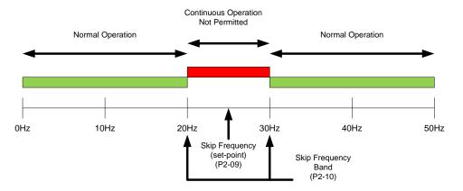
This will give a skip frequency band between 20Hz and 30Hz, centred on 25Hz.
