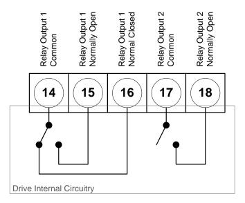
Note that when the drive is powered down, the contacts are always open.
