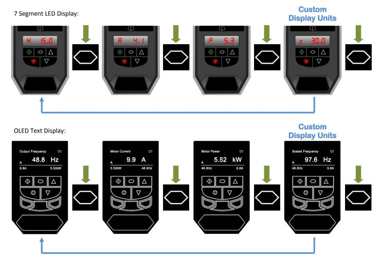
Examples show source (P2-22) set to motor speed and scaling (P2-21) set to 2.000
