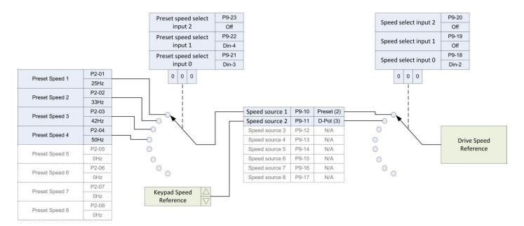
The Following setting should be made to the drive.
