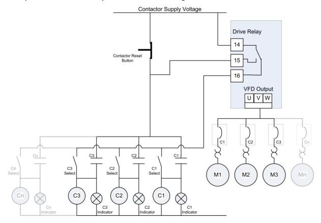
To select a motor the appropriate contactor select switch is closed (C# Select) whilst the drive is disabled. To deselect a motor the appropriate contactor select switch is opened and the contactor reset button pressed whilst the drive is disabled. Selected motors are shown by the corresponding indicators (C# Indicator).
