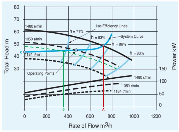
From the curve above, we can see that a single pump operating at maximum speed and the chosen system point produces a flow level of around 720m<sup>3</sup>/h. This is shown by the Red line A. As this point is closest to the optimum pump efficiency, the best system efficiency will be achieved by operating with only one pump up to the maximum flow of a single pump; hence in this case, the Assist Pump Start Speed parameter P8-17 should be close to maximum speed, e.g. 1475 Rpm / 49.9Hz.
