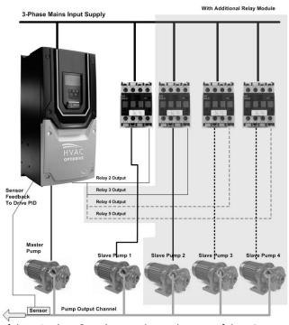
Relay 1 on the standard I/O terminals of the Drive (T14 & T15) cannot be used as part of the DOL control but is freely programmable to other functions through parameter P2-15. Relay 2 on the standard I/O terminals of the Drive (T17 & T18) can be used as the DOL control for the first
