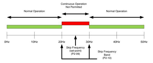
This will give a skip frequency band between 20Hz and 30Hz, centred on 25Hz.
