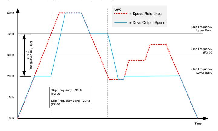
As the speed reference to the Optidrive enters the skip frequency band (either increasing or decreasing speed) the drive output change is frozen at the edge of the skip frequency band until the point that the speed reference crosses the opposing limit. At this point the Optidrive will ramp through the skip frequency band to the opposite limit at the ramp rate specified with the drive ramps.
