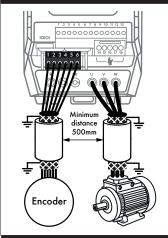
NOTE Do not connect the encoder cable shield to OV of the drive or encoder module.
