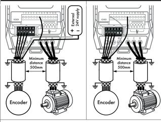
Alternatively (to External supply) the drives on-board 24V supply can be used (T1 (24V) and T7 (OV)) - Ensure total current consumption from T1 does not exceed 100mA.
