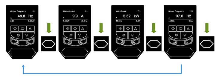
Examples show source (P2-22) set to motor speed and scaling (P2-21) set to 2.000
