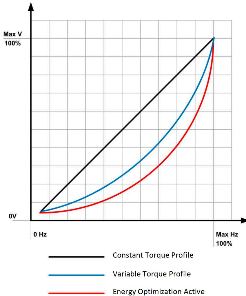
It can be seen that energy savings exist in the area between the different profiles. The Energy Optimization function adjusts voltage to provide energy savings under all conditions. Even a constant torque drive with energy optimization function can operate the motor more efficiently than a variable torque drive without energy optimization.
