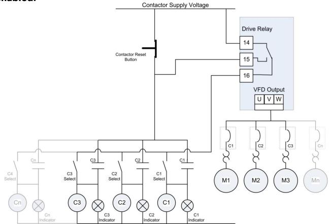
To select a motor, the appropriate contactor select switch is closed (C# Select) whilst the drive is disabled. To deselect a motor, the appropriate contactor select switch is opened and the contactor reset button pressed whilst the drive is disabled. Selected motors are shown by the corresponding indicators (C# Indicator).
