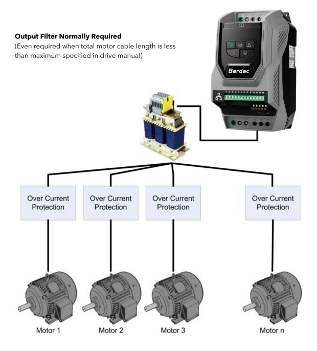
With this connection method individual motor cables are run between the drive and each of the motors with a common connection (star) point located close to the drive. Over-current protection for this configuration is typically located near to the drive so that each motor cable down-stream from the over current protection device is rated only for the motor it protects.
