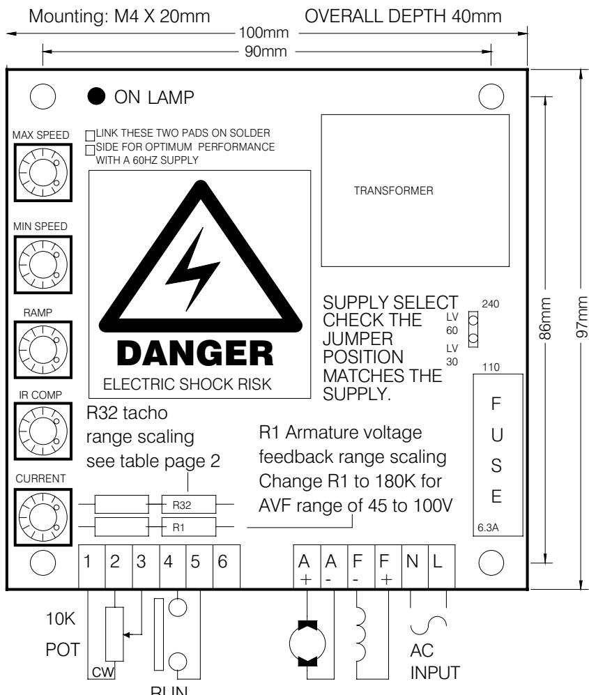
For frequent stopping or jogging it is not good practice to rely on switching the supply off and on to stop and start with the run contact permanently closed. This may result in an uncontrolled current pulse for one half mains cycle under certain conditions. Eg main contact bounce. This could lead to undesired motor movement or device damage. Use a spare NO contact on the main supply contactor in series with T5 and any other RUN contacts in rapid start stop applications
