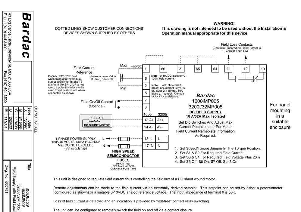
Loss of field current is detected and an indication is provided by "volt-free" contact relay switching.
