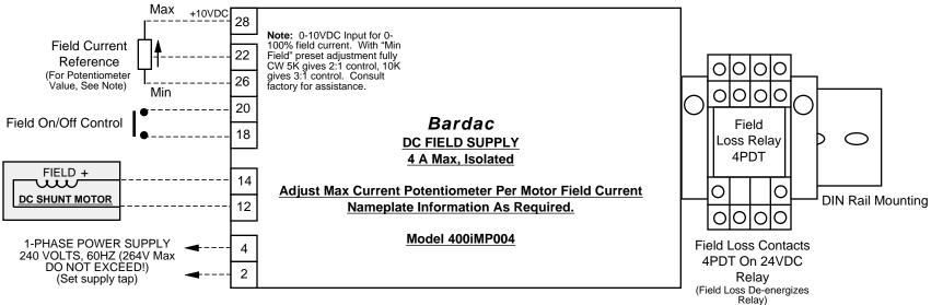
Approximate dimensions: 4"H x 10"L x 3"D For panel mounting in a suitable enclosure
