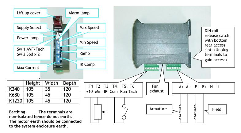
WARNING. This product is non-isolated hence all terminals are at dangerous line potential. Ensure connected items (e.g. speed pot, tach etc.) are not earthed and have sufficient dielectric strength to avoid breakdown. Do not touch any part of the unit. Use an insulated tool to adjust the presets. Do not touch when unit is ON.
