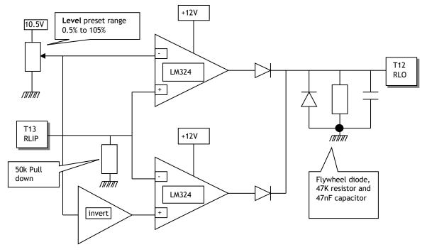
14 **OVLD**. Overload. This output goes high (+10.5V) if the current demand exceeds 110% and the stall timer starts timing. Flywheel diode to COM. See T12 RLOP for details of the output drive capability and configuration.
