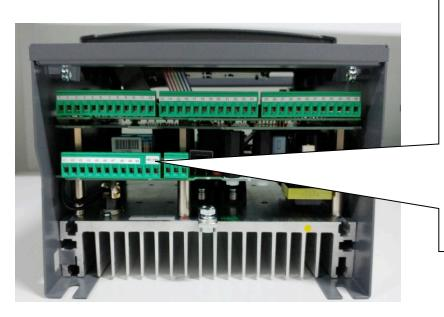
External volt free overtemp switch connected to terminals HS1, HS2.
