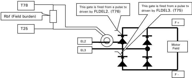
The field current must be sensed by using a current transformer (Acct) on the AC supply to the field bridge. See 7.3 Calibrating an external Field Acct. See also 13 Pulse transformer unit (LA102800), which has provision for mounting Rbf.
