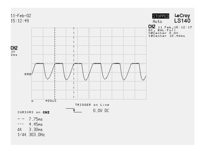
This is a discontinuous current waveform trace using Accts of diameter 150 mm, 4000 turns silicon iron grain orientated steel cores. Notice that there are no turn off tails normally associated with such cores. This is because they have been connected as described.
