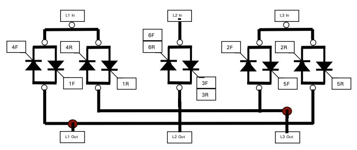
This 4 quadrant configuration saves on 2 thyristors. The 6F and 6R gate outputs must be tied together and used to fire the gate as shown, in the usual way. Similarly the 3F and 3R gate driver outputs must be tied together and used to fire the other gate as shown, in the usual way. The gate outputs are able to be linked because they are open collector.
