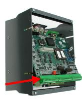
Then, slowly rotate the lower edge of the control board out until the board can be safely slid out of the two upper clips retaining the top of the board.
