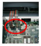
5. With the cover removed, take out the two nylon screws in the lower left and lower right corners of the control board.
