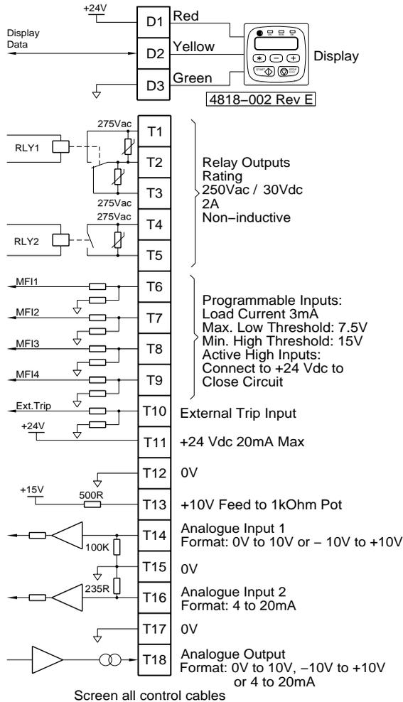
Figure 1.4: The Xtravert Control Inputs and Outputs
