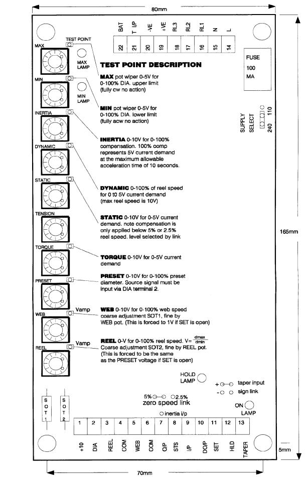
MAX sets the upper limit of diameter detector.
