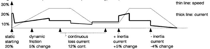
The observations must be made with a full and empty reel. The empty reel is more likely to be used at high speeds and the full reel at low speeds. The purpose of these observations is to find out how much current will be used to overcome the losses and hence be unavailable to provide tension in the web. A system with low losses will be the most accurate. A system with high losses and low tension requirement will be the least accurate.
