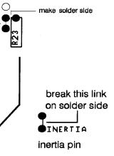
ZERO SPEED THRESHOLD With large build up ratios and reduced web speeds, the reel speed can easily become less than the 2.5% threshold. (eg 10 : 1 build up at 25% web speed = 2.5% reel speed). To reduce the threshold below 2.5%, remove the jumper and connect an externally generated voltage signal to the centre pin of the selector. The voltage level required is 100mV per % threshold. Note, the calculation accuracy is reduced below the standard threshold.
