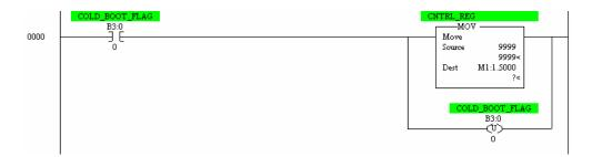
If the module will be sending event messages to the module to execute on the Ethernet port to other nodes on the network, the following rung may be used:
