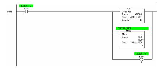
When the event flag is set, data in the event file is transferred to the module in using a control code of 2000. When the module receives the block, it places the event in the command queue. This is a simple means to send user-generated commands to any node on the network. A file of event commands can exist as a static or dynamic list and can be executed under control of user ladder logic. Make sure that the block is compatible with the *Event Command Block* (on page 10).
