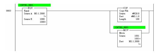
Use this feature to initialize the output data in the module with the values currently held in the processor. This feature is employed to bring the output data to a known or last set state.
