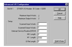
The next step in the module's setup is to define the user-defined data areas to hold the status and read and write database areas. Edit the BARDACDW.CFG file now for the application to implement. Use any text editor to set the values in the file. You must retain the file name BARDACDW.CFG.
