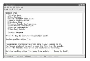
4 From the **Transfer** menu in HyperTerminal, select **Receive File**. This action opens the Receive File dialog box.
