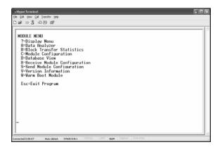
2 Press [S] (Send Module Configuration). The message "Press Y key to confirm configuration send!" is displayed at the bottom of the screen.
