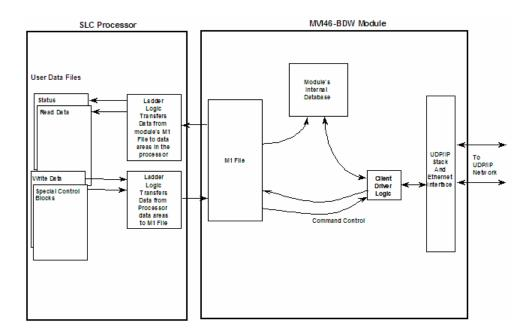
As shown in the diagram above, all data transferred between the module and the processor over the backplane is through the M1 file. Ladder logic must be written in the SLC processor to interface the M1 file data in the module's internal database. All data used by the module is stored in its internal database. This database is defined as a virtual data table with addresses from 0 (40001) to 4999 (45000). The following illustration shows the layout of the database:
