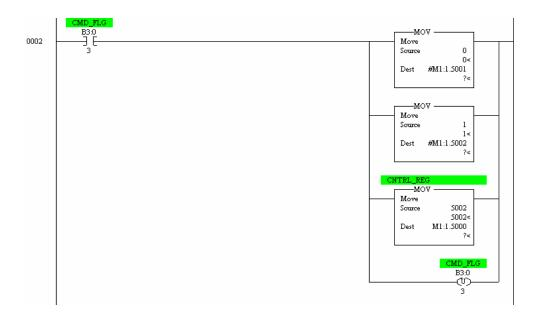
If the module is configured to receive the processor data set on startup, the following rung is required:
