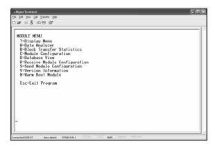
**2** Press **[S]** (Receive Module Configuration). The message "Press Y key to confirm configuration receive!" is displayed at the bottom of the screen.
