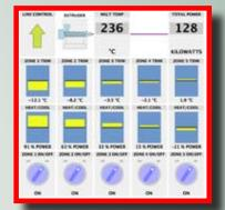
**Total Control** Touch the TEMP CONTROL tile to drill down to the heater controllers. Touch the MELT TEMP tile to set the master temperature setpoint.
