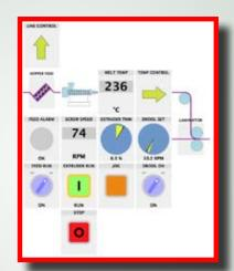
Operator Screen Touch a graphic tile to drill down to the detail screen
